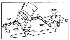
HotchKiss' revolutionary frame design. Drawing at left shows details of the cast frame and the rear subframe; drawing above shows how body was mounted on these components
